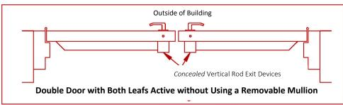
This application is compatible with *concealed vertical rod exit devices*. "E" swing on order form swing chart.
